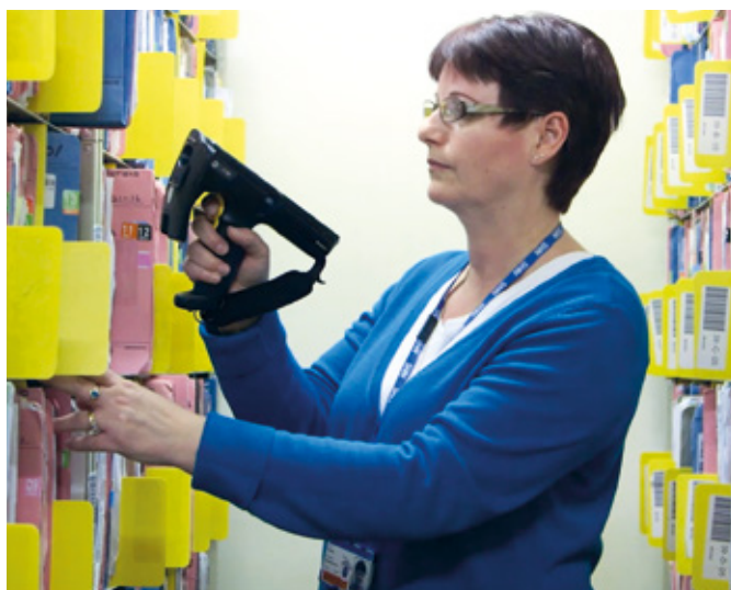
Location based filing: a file's physical location is digitally recorded by scanning its barcode and its destination during pull and put away.
